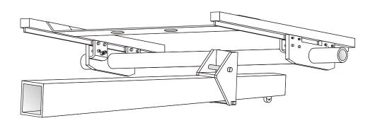
The underbody clamp secures to the pinch welds allow more versatile positioning of the body straightener.
