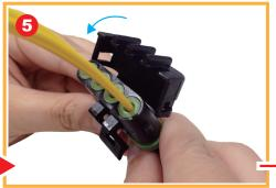
Once all terminals are inserted lock wire and seals as shown above.
