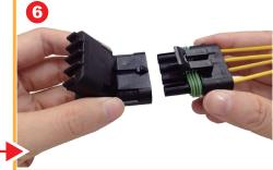
Once all terminals are inserted, Connect together until locked.
