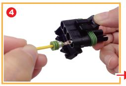
Insert crimped Weather Pack Terminal into connector housing.
